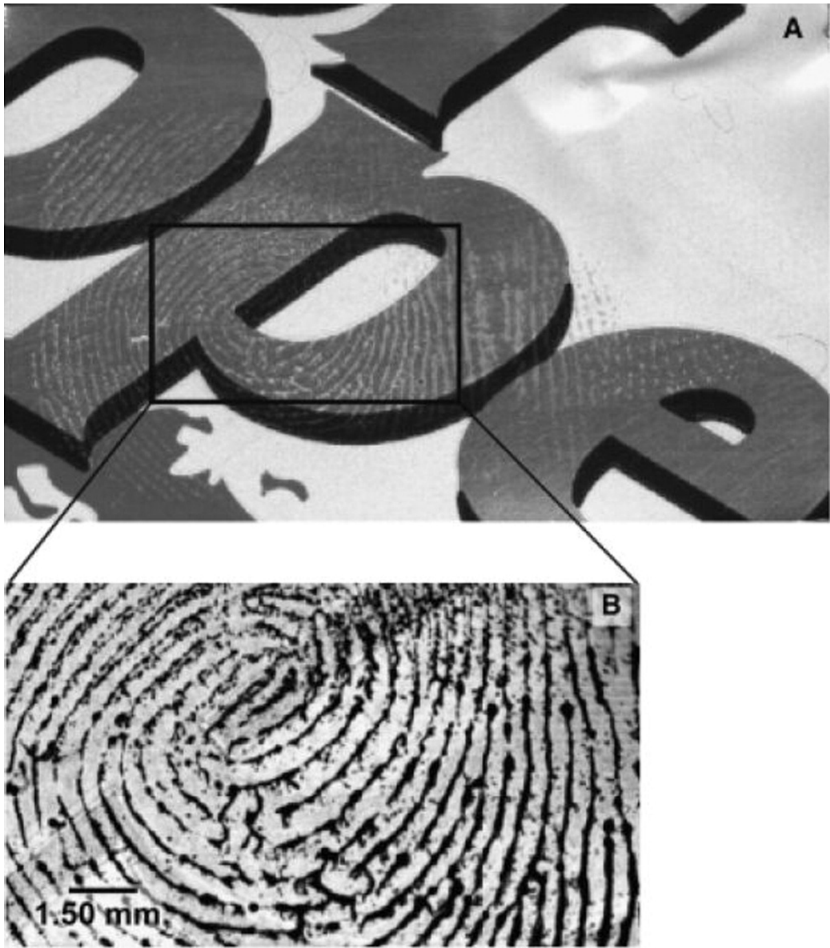
Figure 1.1: Cut and flattened Dr. Pepper soda can with a deposited fingerprint. (A) The soda can be imaged using a document scanner. (B) An infrared image of the highlighted area was generated by mapping the band intensity at 9842 nm. Adapted from [Crane et al., 2007].
