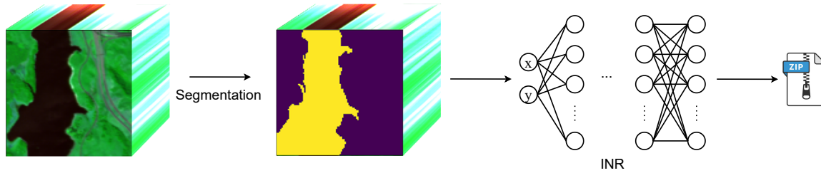
Figure 1.7: Overview of the proposed task-aware hyperspectral image compression method. The approach consists of two stages: segmentation and selective compression. In the segmentation stage, K-means clustering is used to identify regions of interest (ROI) based on the task requirements. During the compression stage, the segmented regions are compressed with higher fidelity to preserve critical spectral information, while background areas are compressed with less stringent criteria to optimize overall compression efficiency.
