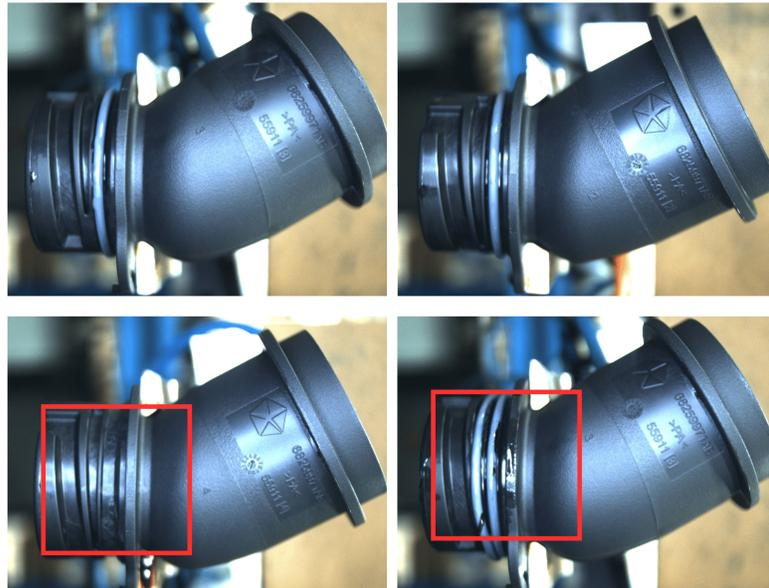
Figure 5.4: Example samples from the Axiom dataset. The first row shows normal samples produced by the injection molding machine, and the second row shows defective samples.
