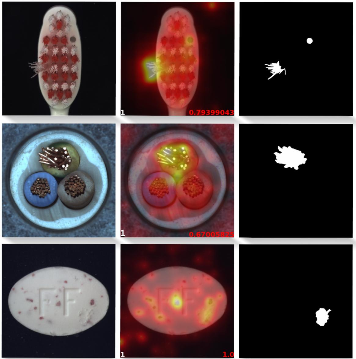
Figure 5.6: Visualization results from MVTec [5] dataset. The first column shows the input image, the second column shows the generated heatmap along with the prediction score at the bottom and the last column shows the ground truth pixel labels.
