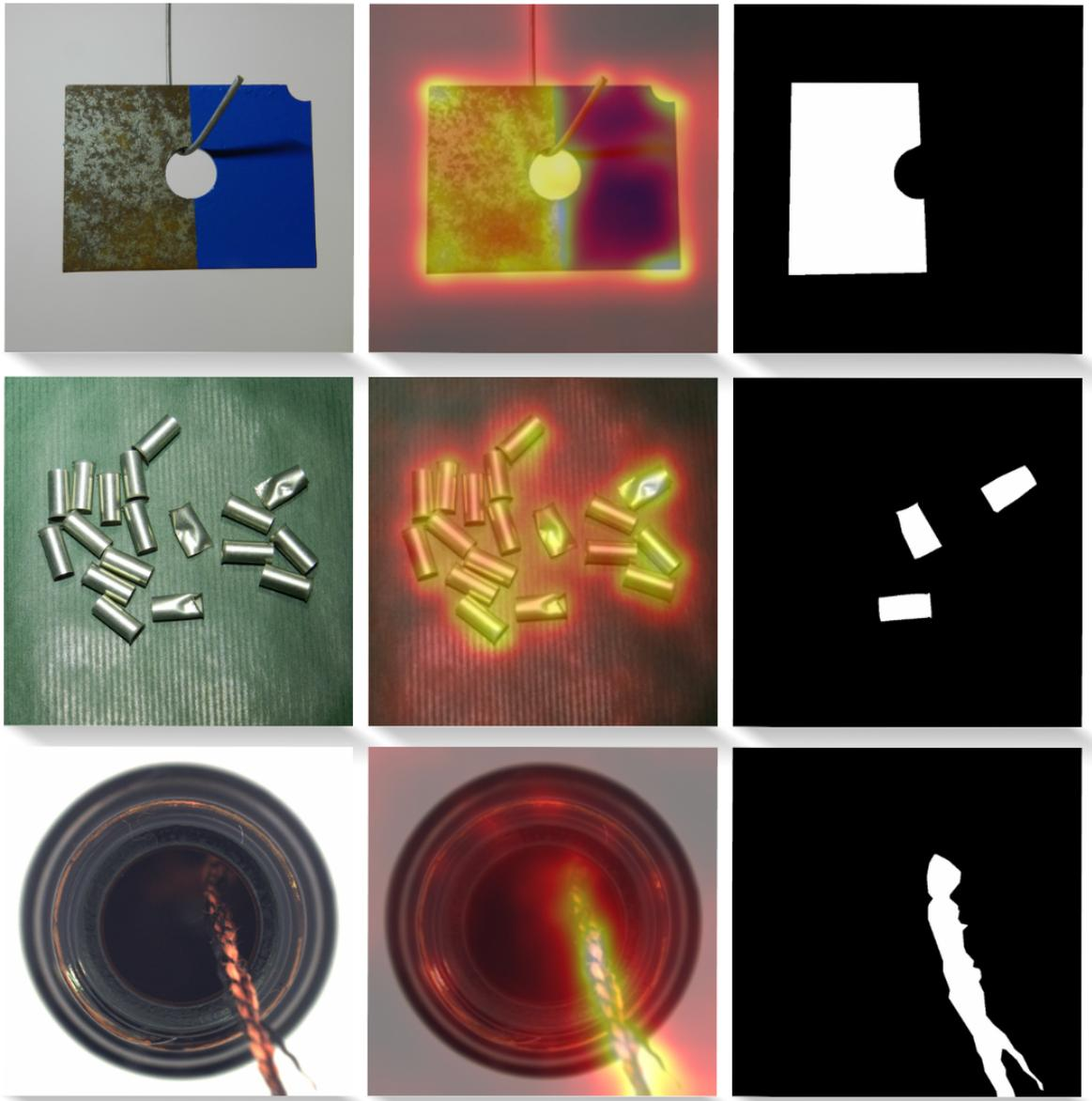
Figure 5.5: Visualization results from MPDD [31] dataset. The first column shows the input image, the second column shows the generated heatmap and the last column shows the ground truth pixel labels.
