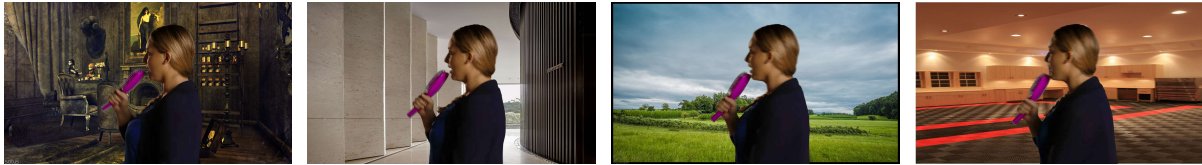
Figure 5.1: Showcasing Background Shuffling in Dataset: This figure consists of four frames from our dataset, illustrating the technique of background shuffling. Each frame features the same foreground subject from one video, set against a different background.
