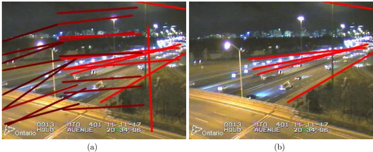
Figure 5.7: Estimated quality for different clusters accumulated from 25 frames: (a) mean of clusters with around 20 line segments; (b) mean lines of clusters with around 60 segments. Increased colour intensity indicates high cluster confidence.
