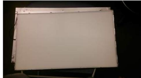
(d) The removed backlight from the front LCD.
