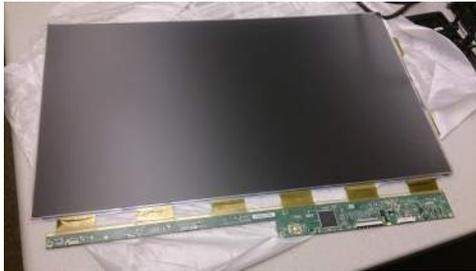
(c) The front LCD after removed from the original monitor.
