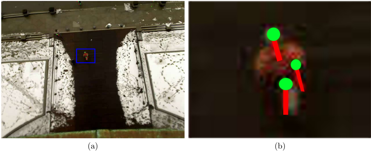
Figure 3.1: Sparse inter-frame motion vectors for pixels corresponding to a single pedestrian (left). The right image shows a closeup view of the region bounded by the blue rectangle. Green circles indicates arrow heads.
