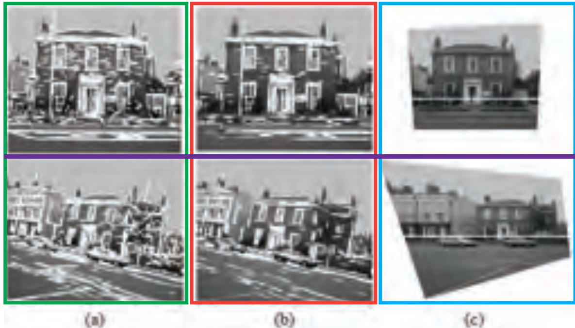
Figure 2.3: Obtaining a canonical view in [Robertson and Cipolla, 2004]. (a) Straight line segments are detected from an image. (b) After filtering, line segments associated with horizontal and vertical vanishing points are kept. (c) The image is transformed into a canonical frame using a rectified view of the dominant plane. Image courtesy of [Robertson and Cipolla, 2004]
